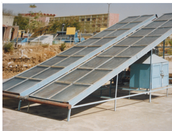
Plate. 3. Solar drier with forced convection
