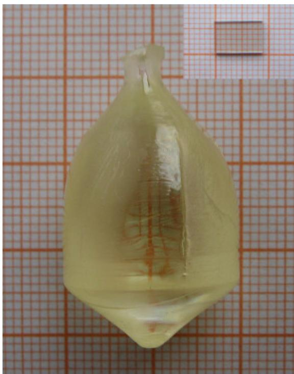
Fig. 1. A  $\text{Yb}^{3+}:\text{Li}_2\text{Gd}_4(\text{MoO}_4)_7$  crystal grown by the Czochralski method
