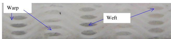
Fig. 3. Cross-section of the 2.5D braided CMCs
