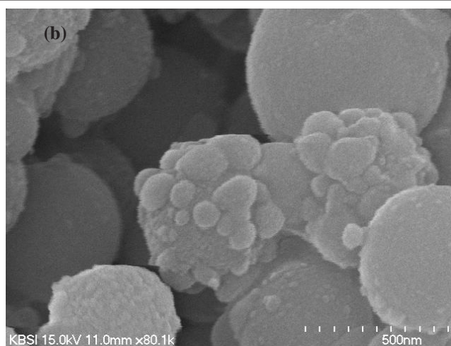
Fig. 2. SEM images of (a) silica-silver nanocomposites with APTMS linkers and (b) silica-silver nanocomposites with MPTMS linkers
