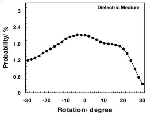
Fig. 3. Variation of probability with respect to rotation about x-axis during stacking interactions at room temperature (300 K)
