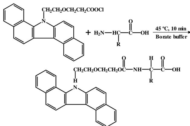
Fig. 1. Derivatization scheme of DBCEC with amino acids
