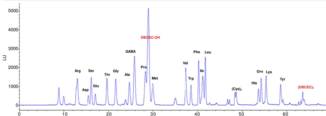
Fig. 2. Chromatogram of the standard amino acid derivatives with DBCEC
