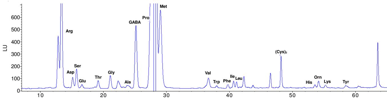
Fig. 3. Chromatogram for the analysis of free amino acid derivatives from the extracted *H. rhamnoides* L. fruit samples
