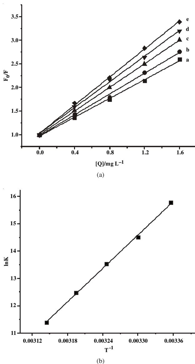
Fig. 6. (A) The Stern-Volmer plot for the binding of 1,4-DHAQ with OFL at 298 K (a), 303 K (b), 308 K (c), 313 K (d) and 318 K (e). (B) Van't Hoff plot for the binding of 1,4-DHAQ with OFL
