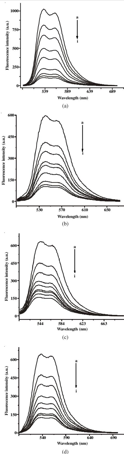
Fig. 3. Quenching effect of OFL (A), NOR (B), CIP (C) and GAT (D) on 1,4-DHAQ.  $\lambda_{ex} = 484$  nm, A:  $20 \text{ mg L}^{-1}$  of 1,4-DHAQ, B, C and D:  $10 \text{ mg L}^{-1}$  of 1,4-DHAQ. a  $\rightarrow$  i: 0.0, 0.4, 0.8, 1.2, 1.6, 2.0, 2.4, 2.8,  $3.2 \text{ } \mu\text{g mL}^{-1}$  OFL (A), NOR (B), CIP (C) and GAT (D)
