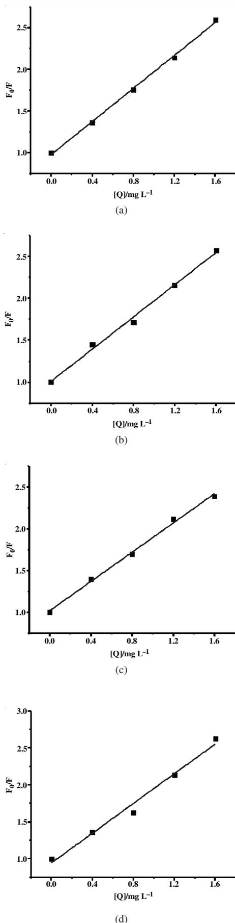
Fig. 4. Linear Stern-Volmer plots of fluorescence quenching of 1,4-DHAQ by OFL (a), NOR (b), CIP (c), and GAT (d) at 298 K
