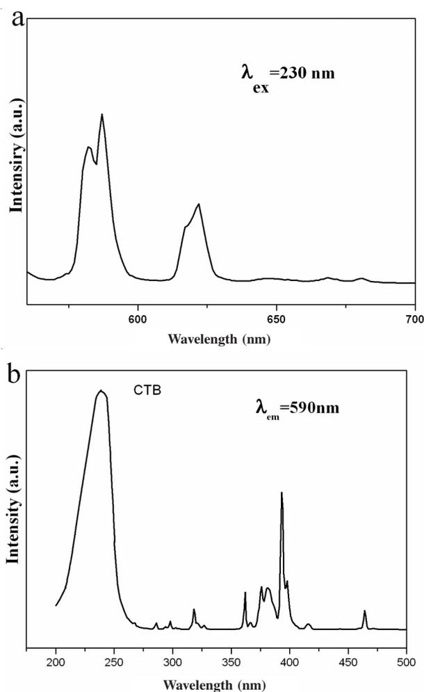
Fig. 3. Excitation spectra (a) and emission spectra (b) of the  $\text{YPO}_4:\text{Eu}^{3+}$  cornflakes
