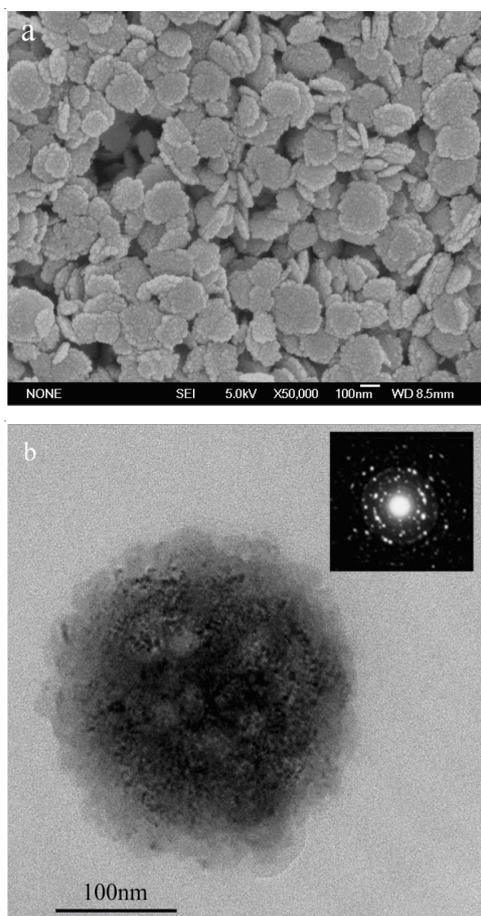
Fig. 2. SEM image (a), TEM image and SEAD pattern (b) of  $\text{YPO}_4:\text{Eu}^{3+}$  cornflakes
