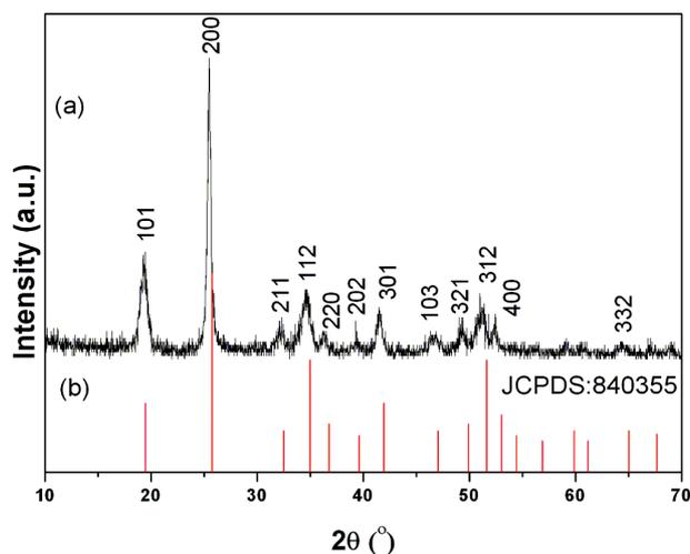
Fig. 1. XRD pattern for the  $\text{YPO}_4:\text{Eu}^{3+}$  cornflakes
