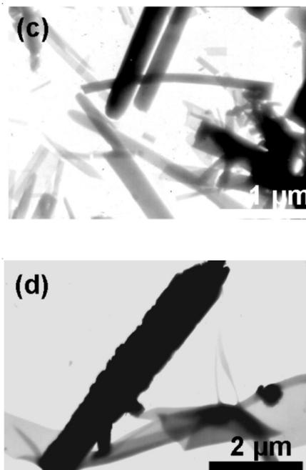
Fig. 2. TEM images of Dy-BDC in the presence of CTAB for various reaction times: (a) 10, (b) 30, (c) 180, (d)
