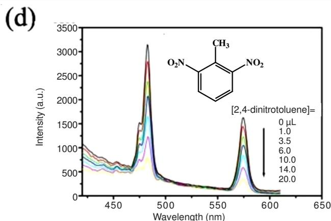
Fig. 3. Variation of emission spectra of Dy-BDC nanorods with the volume of 0.78 M of nitroaromatics (a) 2-NT, (b) 4-NT, (c) 2,4-DNT and (d) 2,6-DNT in 2 mL of acetonitrile
