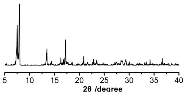
Fig. 1. Powder XRD patterns of Dy-BDC nanocrystals
