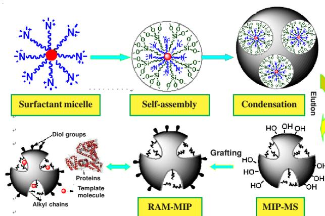
Fig. 1. Synthesis protocol of restricted access materials-molecularly imprinted polymers
