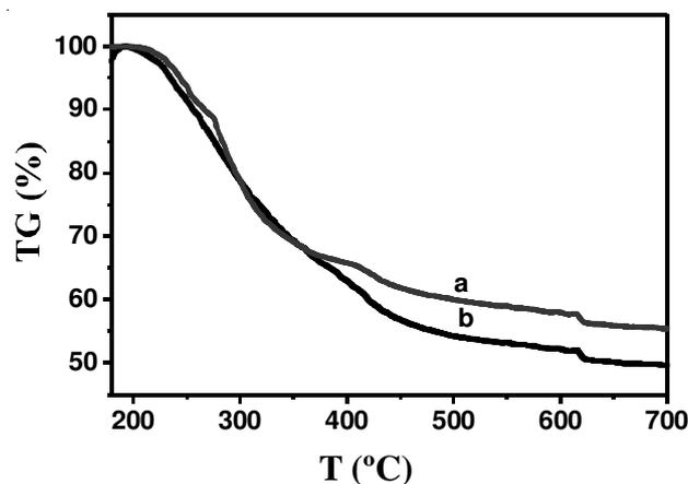
Fig. 3. TG curves of MIP-MS (a) and RAM-MIP (b)
