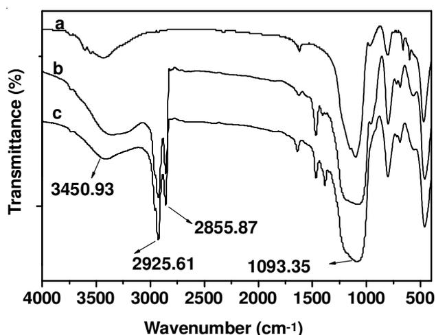
Fig. 2. FT-IR spectra of  $\text{SiO}_2$  (a), MIP-MS (b) and RAM-MIP (c)
