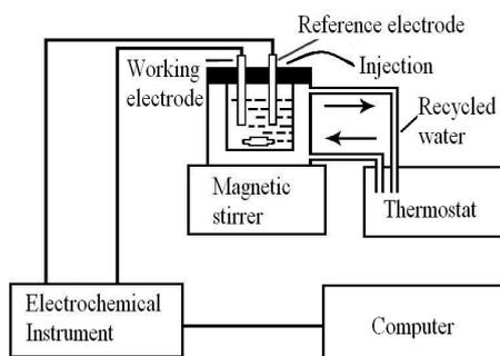
Fig.1. Scheme of Belousov-Zhabotinskii (B-Z) oscillation device
