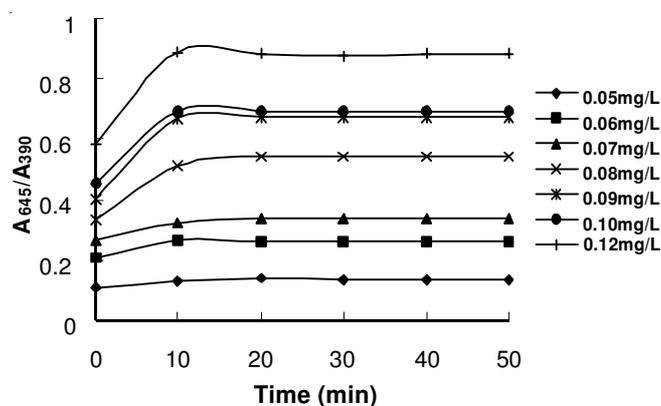
Fig. 5. Time-dependent absorbance changes upon the interaction between modified silver nanoparticles and 5-fluorocytosine target in the concentration range of 0.05-0.12 mg/L
