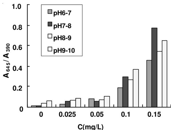
Fig. 7. pH-dependent colourimetric analysis of 5-fluorocytosine using modified silver nanoparticles
