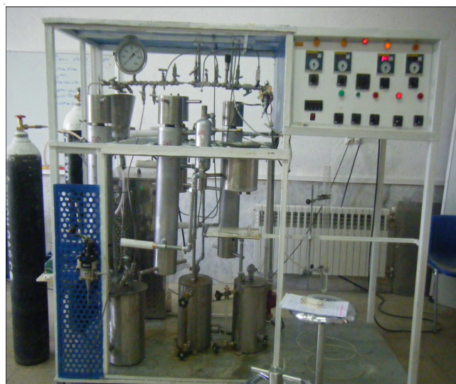
Fig. 4. Laboratory extraction system by supercritical fluid technology
