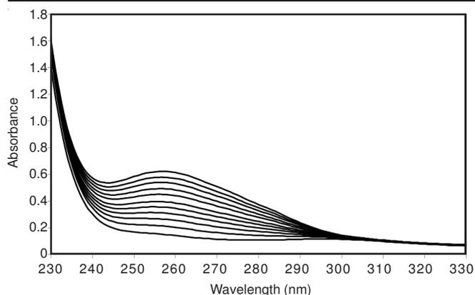
Fig. 4. Absorption spectra of Bi(III)-myricetin in different concentrations of ds-DNA.  $C_{\text{DNA}} = 0.0, 6.1, 12.2, 18.3, 24.4, 30.5, 36.6, 42.7, 48.8, 54.9, 60.3$  and  $61.0 \mu\text{mol L}^{-1}$  for curves 1-12,  $C_{\text{Bi(III)}} = 10.0 \mu\text{mol L}^{-1}$ ,  $C_{\text{myricetin}} = 10.0 \mu\text{mol L}^{-1}$  in phosphate buffer ( $0.02 \text{ mol L}^{-1}$ , pH 7.5)
