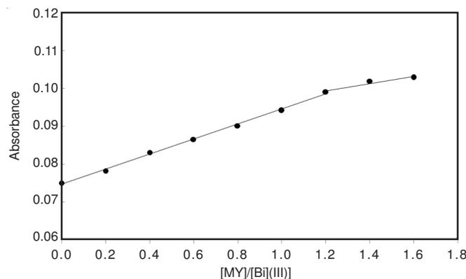
Fig. 3. Mole ratio plot of myricetin in presence of Bi(III) at different concentrations. Conditions: [Bi<sup>3+</sup>] = 0, 2.0, 4.0, 6.0, 8.0, 10.0, 12.0, 14.0 and 16.0  $\mu\text{mol L}^{-1}$ ,  $C_{\text{myricetin}} = 10.0 \mu\text{mol L}^{-1}$ , phosphate buffer (0.02 mol L<sup>-1</sup>, pH 7.5)
