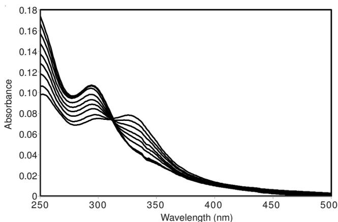
Fig. 2. Absorption spectra of myricetin in presence of Bi(III) at different concentrations. Conditions: [Bi<sup>3+</sup>] = 0, 2.0, 4.0, 6.0, 8.0, 10.0, 12.0, 14.0 and 16.0  $\mu\text{mol L}^{-1}$  for curves 1-9 and  $C_{\text{myricetin}} = 10.0 \mu\text{mol L}^{-1}$ , phosphate buffer (0.02 mol L<sup>-1</sup>, pH 7.5)
