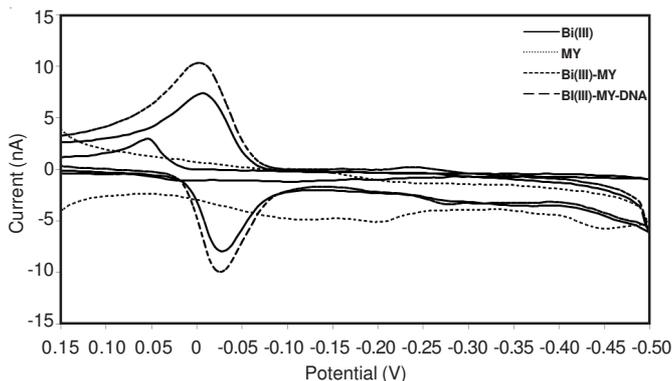
Fig. 7. Cyclic voltammetry of Bi(III), myricetin, Bi(III)-myricetin complex and Bi(III)-myricetin in the presence of ds-DNA on the surface of HMDE. Conditions:  $C_{\text{Bi(III)}} = 20.0 \mu\text{mol L}^{-1}$ ,  $C_{\text{myricetin}} = 10.0 \mu\text{mol L}^{-1}$ ,  $C_{\text{DNA}} = 9.2 \mu\text{mol L}^{-1}$ ,  $v = 50.0 \text{ mV s}^{-1}$ , pulse amplitude 2.0 mV, phosphate buffer ( $0.002 \text{ mol L}^{-1}$ , pH 7.5)
