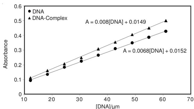
Fig. 5. Calibration curves for ds-DNA in the absence and presence of Bi(III)-myricetin at 260 nm. Conditions: phosphate buffer ( $0.002 \text{ mol L}^{-1}$ , pH 7.5),  $C_{\text{myricetin}} = 10 \mu\text{mol L}^{-1}$ ,  $C_{\text{Bi(III)}} = 10 \mu\text{mol L}^{-1}$
