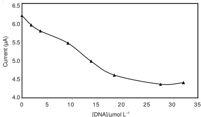
Fig. 8. Binding curve of Bi(III)-myricetin complex at different concentrations of ds-DNA.  $C_{\text{ds-DNA}} = 0.0, 1.8, 3.7, 9.2, 13.7, 18.3, 27.5$  and  $32.1 \mu\text{mol L}^{-1}$ .  $C_{\text{Bi(III)}} = 30.0 \mu\text{mol L}^{-1}$  and  $C_{\text{myricetin}} = 20.0 \mu\text{mol L}^{-1}$  in phosphate buffer ( $0.002 \text{ mol L}^{-1}$ , pH 7.5),  $v = 50 \text{ mV s}^{-1}$ , pulse amplitude 2 mV
