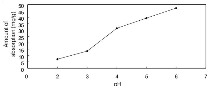
Fig. 4. Effect of pH on adsorption of Pb(II)
