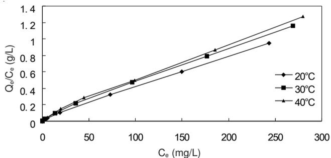
Fig. 6. Langmuir plots for tremolite amianthus adsorption
