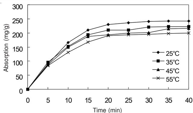
Fig. 3. Effect of contact time on the adsorption of  $Pb(II)$  on tremolite amianthus at various temperatures
