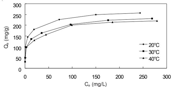
Fig. 5. Adsorption isotherms for tremolite amianthus
