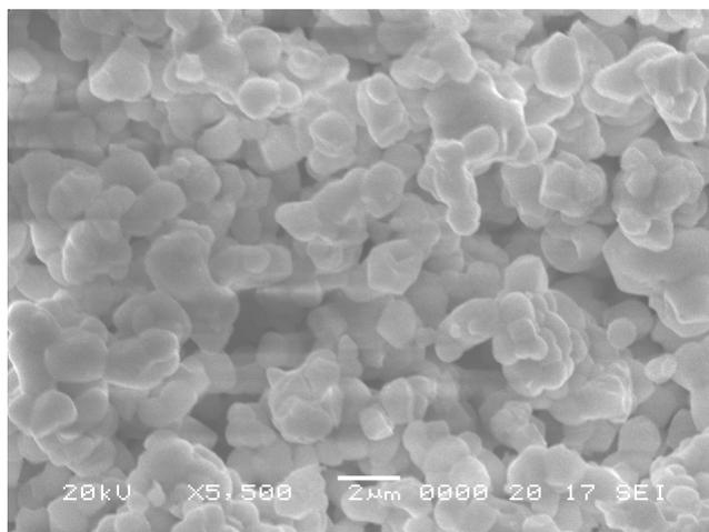
Fig. 2. SEM image of the  $\text{CaWO}_4$  particles after solid-state metathetic reaction followed by heat-treatment at 600 °C for 3 h
