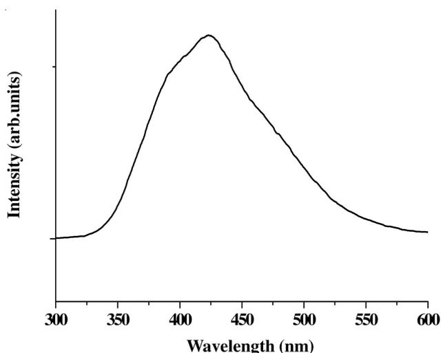
Fig. 4. Photoluminescence emission spectra of the  $\text{CaWO}_4$  particles excited at 240 nm at room temperature
