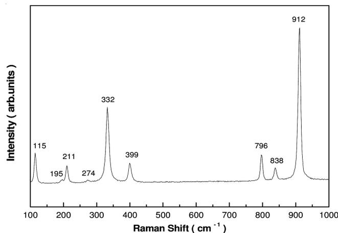
Fig. 5. Raman spectra of the  $\text{CaWO}_4$  particles excited by the 514.5 nm line of an Ar-ion laser at 0.5 mW on the sample
