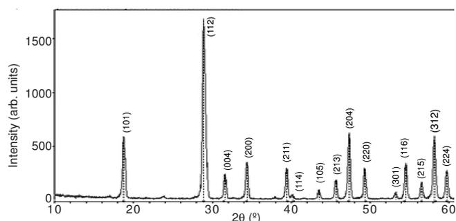
Fig. 1. XRD patterns of the  $\text{CaWO}_4$  particles after solid-state metathetic reaction followed by heat-treatment at 600 °C for 3 h
