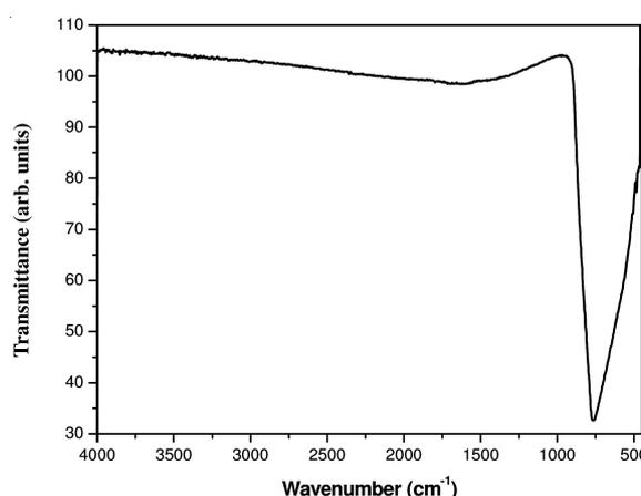
Fig. 3. FT-IR spectra of the  $\text{CaWO}_4$  particles after solid-state metathetic reaction followed by heat-treatment
