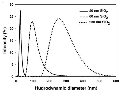
Fig. 5. Size distribution of 20, 60 and 238 nm SiO<sub>2</sub> nanoparticles obtained by DLS
