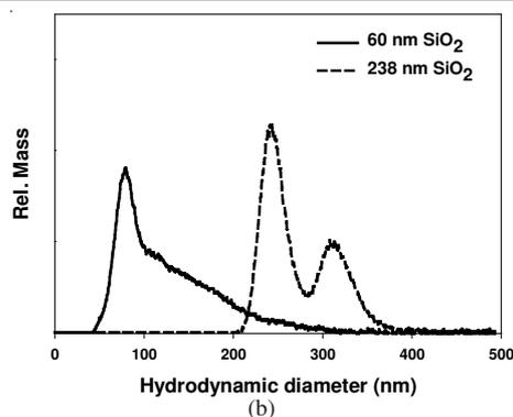
Fig. 4. AsFIFFF fractograms (a) and size distributions (b) of SiO<sub>2</sub> nanoparticles having nominal mean diameters of 60 and 238 nm overlaid. Flow rate were  $F_{out} = 1.02$  and  $F_c = 0.52$  mL/min. The carrier liquid was the same as that used in Fig. 1
