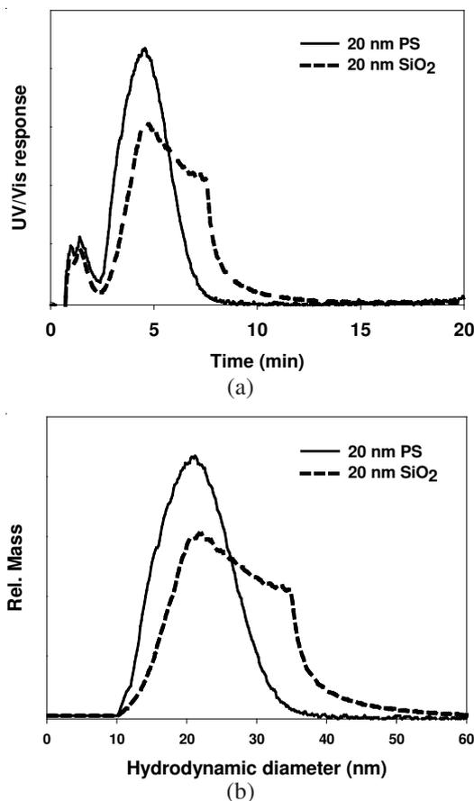
Fig. 2. AsFIFFF fractograms (a) and size distributions (b) of polystyrene latex beads and SiO<sub>2</sub> nanoparticles having nominal mean diameters of 20 nm. Flow rate were  $F_{out} = 0.52$  and  $F_c = 1.52$  mL/min. The carrier liquid was the same as that used in Fig. 1
