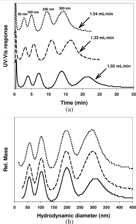
Fig. 1. AsFIFFF fractograms (a) and size distributions (b) of a mixture of four polystyrene latex beads obtained at various channel flow rate ( $F_{out}$ ).  $F_c$  was fixed at 0.52 mL/min. The carrier liquid was water containing 0.1 % FL-70 and 0.02 % NaN<sub>3</sub>.
