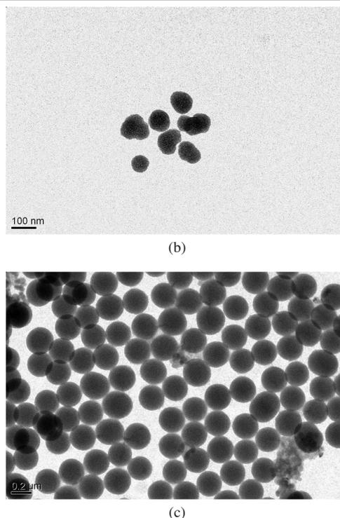
Fig. 3. TEM images of SiO<sub>2</sub> nanoparticle having nominal diameters of 20 (a), 60 (b) and 238 nm (c)
