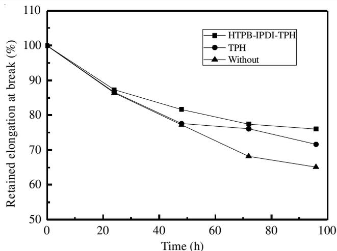
Fig. 6. Retained elongation at break of natural rubber vulcanizates at different time after water extraction
