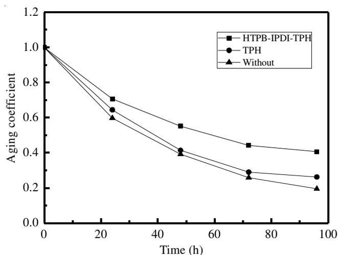
Fig. 7. Aging coefficient (K) of natural rubber vulcanizates at different time after water extraction
