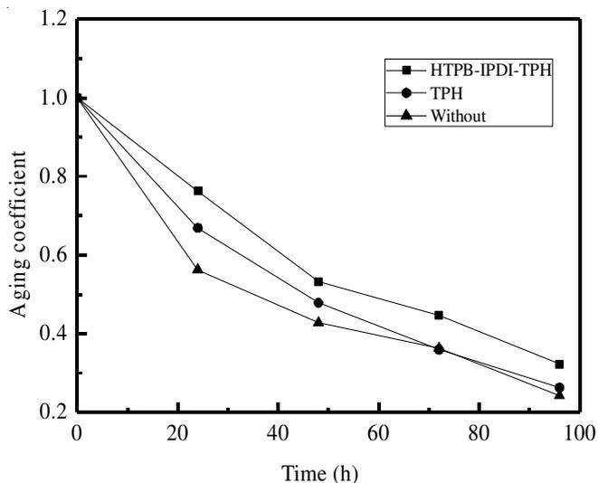
Fig. 4. Aging coefficient (K) of natural rubber vulcanizates at different time after methanol extraction
