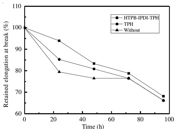
Fig. 3. Retained elongation at break of natural rubber vulcanizates at different time after methanol extraction
