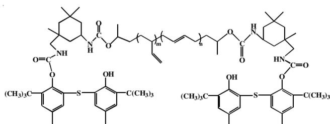
Fig. 1. Structure of HTPB-IPDI-TPH
