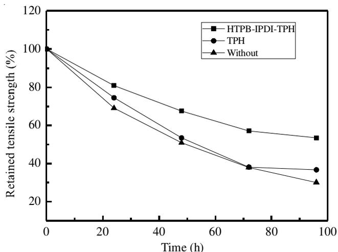
Fig. 5. Retained tensile strength of natural rubber vulcanizates at different time after water extraction
