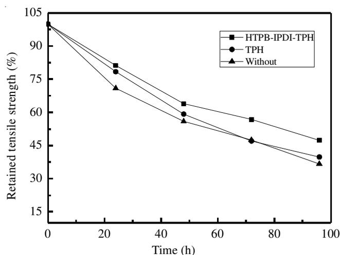
Fig. 2. Retained tensile strength of natural rubber vulcanizates at different time after methanol extraction
