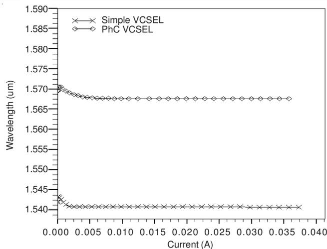
Fig. 4. Optical wavelength for the vertical cavity surface emitting lasers (VCSELs) with various structures
