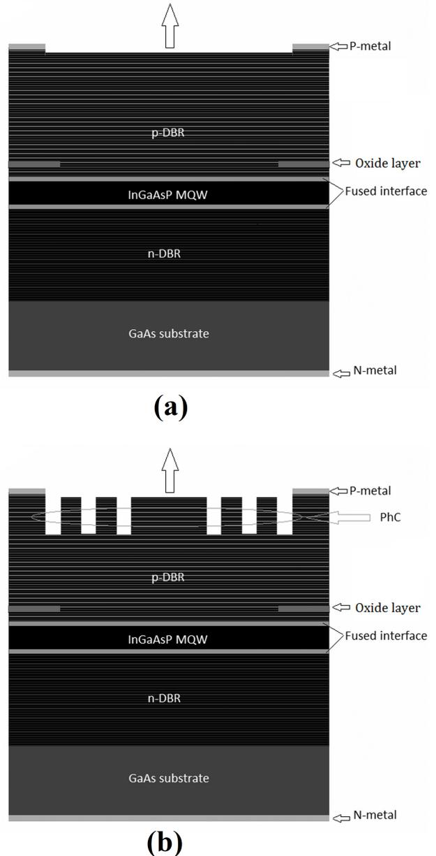
Fig. 2. Schematic structure of the laser devices (a) Simple vertical cavity surface emitting laser (b) PhC vertical cavity surface emitting laser
