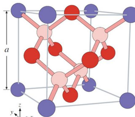
Fig. 1. Ball-and-stick (atomic) representation of several three-dimensional lattices in a cubic supercell, with a lattice constant  $a$ . The blue balls alone form a simple cubic lattice. Adding the dark red balls produces a face-centered cubic (fcc) lattice. Adding the pink balls as well produces a diamond lattice, with stick bonds (four bonds per ball)
