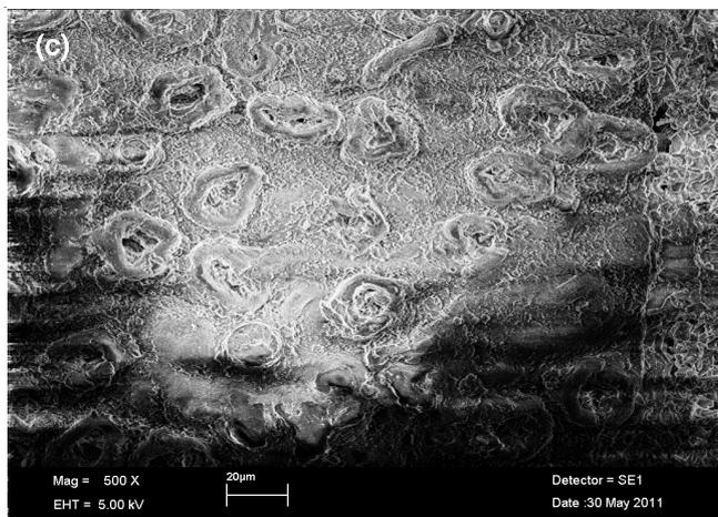
Fig. 1(c). SEM Micrograph of Banyan tree leaves after adsorption of methylene Blue
