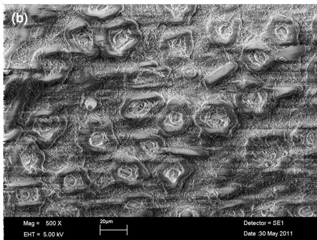
Fig. 1(b). SEM Micrograph of Banyan tree leaves after adsorption of malachite green
