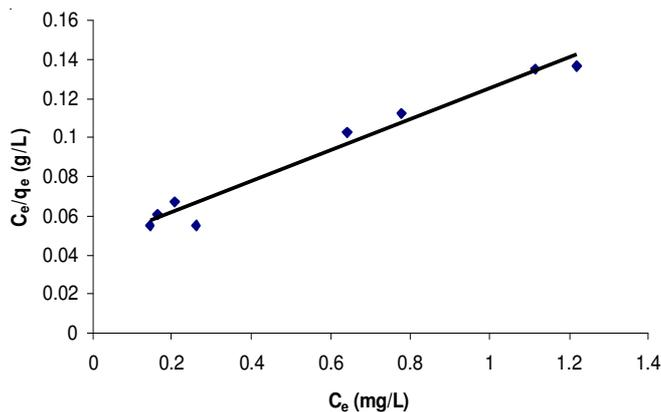
Fig. 3. Langmuir isotherm for the adsorption of malachite green on Banyan leaves
