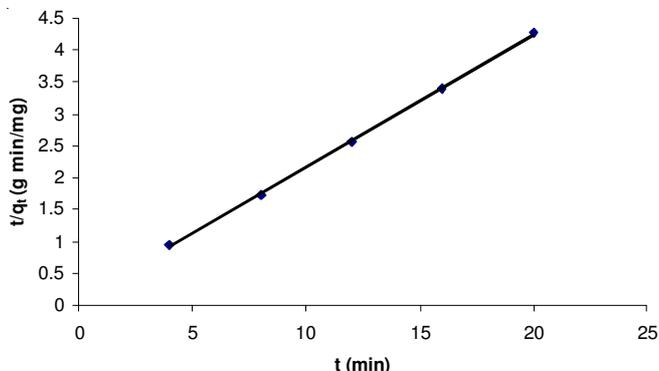
Fig. 5. Plot for pseudo second order kinetic model for the adsorption of malachite green on Banyan leaves
