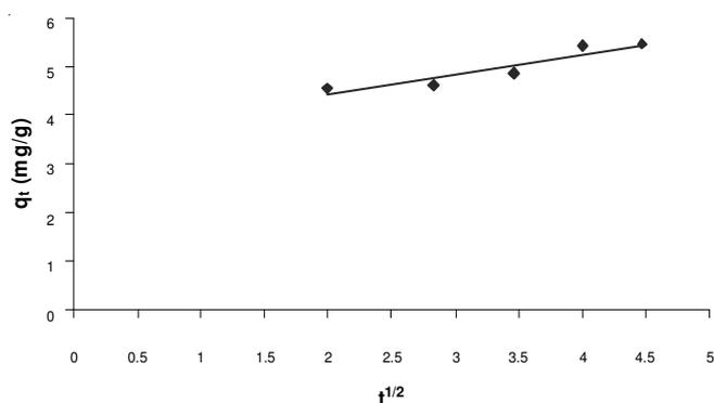
Fig. 7. Plot of intraparticle diffusion model for the adsorption of malachite green on Banyan leaves
