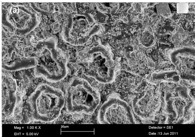
Fig. 1(a). SEM Micrograph of Banyan tree leaves before adsorption
