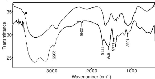
Fig. 1. FTIR spectra of (a) Chitosan and (b) Chitosan-g-poly(NaAA-co-AN)
