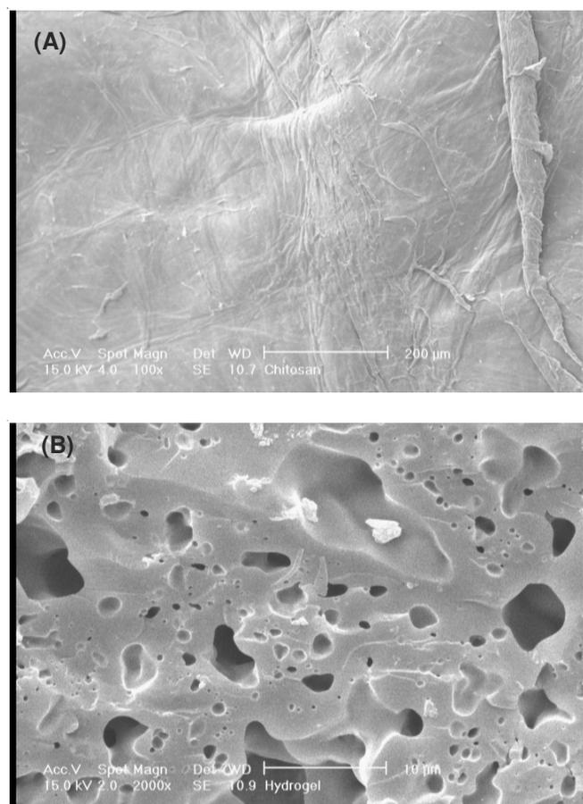
Fig. 2. SEM photograph of Chitosan (A) and the optimized super absorbent hydrogel (B)
