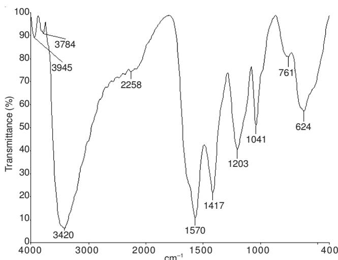
Fig. 4. FTIR spectrum of Congo red crystal
