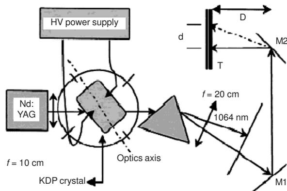
Fig. 7. Experimental setup for second harmonic generation measurement
