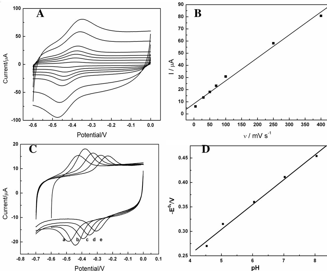
Fig. 2. (A) Cyclic voltammograms of the GOD/IL-GNs/GC electrode in PBS with  $\text{N}_2$ -saturated at various scan rate. (B) The plots of peaks vs. scan rates. (C) Cyclic voltammograms of the GOD/IL-GNs/GC electrode in PBS with  $\text{N}_2$ -saturated at various pH, from a to e the pH value is 4.5, 5.0, 6.0, 7.0 and 8.0. (D) The plots of peaks vs. pH value
