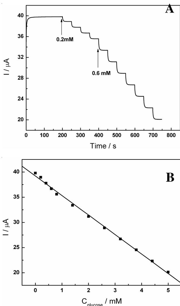
Fig. 3. (A) Typical steady-state current response of the biosensor on successive addition of glucose. Applied potential, -0.5 V. (B) Calibration curve of the electrocatalytic current on the concentration of glucose
