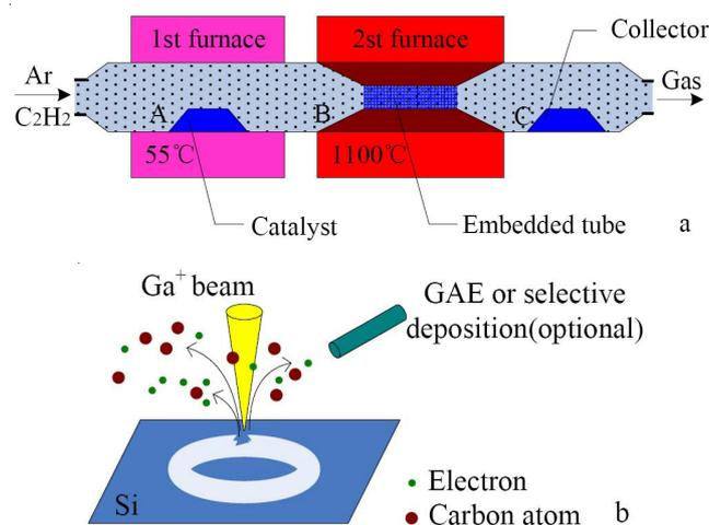
Fig. 2. Schematic diagrams of the apparatus used for synthesizing toroidal carbon nanotubes (a) and processing toroidal carbon nanotubes to coiled carbon nanotubes (b)
