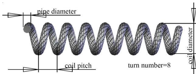
Fig. 1. Structural parameters of coiled carbon nanotubes
