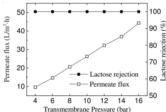
Fig. 10. Variation of permeate flux and lactose rejection with transmembrane pressure in the nanofiltration membrane (Feed flow rate = 1680 l/h, temperature = 30-35 °C, feed COD = 570 mg/L, feed flow rate = 1440 l/h)
