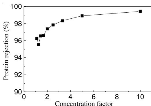
Fig. 9. Protein rejection as a function of concentration factor in the ultrafiltration membrane (Transmembrane pressure = 10 bar, feed flow rate = 1920 l/h, temperature = 30-35 °C, feed COD concentration = 3000 mg/L)
