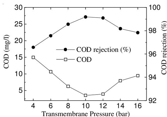
Fig. 11. Variation of COD and COD rejection with transmembrane pressure in the nanofiltration membrane (Feed flow rate = 1680 l/h, temperature = 30-35 °C, feed COD concentration = 570 mg/L)
