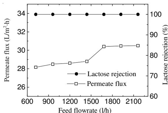
Fig. 12. Variation of permeate flux and lactose rejection with feed flow rate in the nanofiltration membrane (Transmembrane pressure = 10 bar, temperature = 30-35 °C, feed COD concentration = 570 mg/L)
