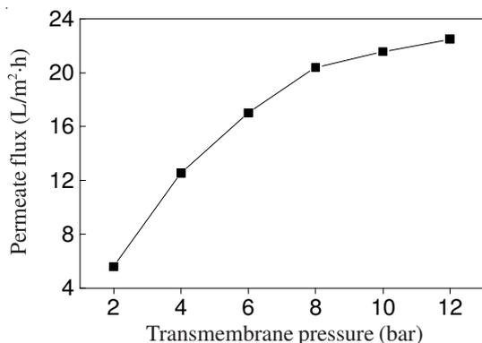
Fig. 3. Pure water flux as a function of transmembrane pressure for three different flow rates (Q) in the nanofiltration membrane
