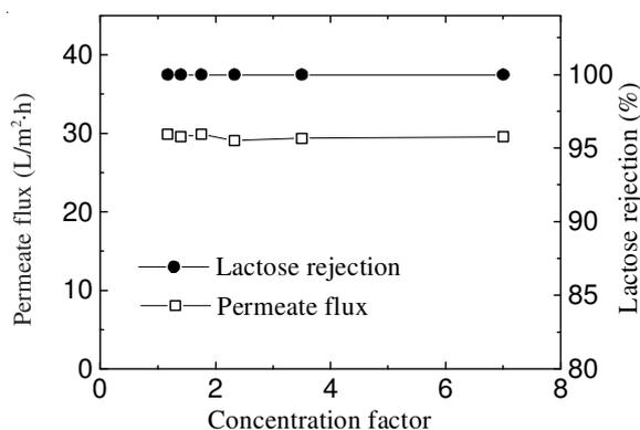
Fig. 14. Variation of permeate flux and lactose rejection with concentration factor in the nanofiltration membrane (Transmembrane pressure = 10 bar, feed flow rate = 1680 L/h, temperature = 30-35 °C, feed COD concentration = 570 mg/L).
