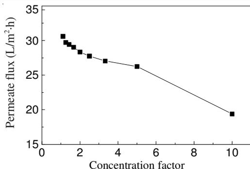
Fig. 8. Permeate flux variation as a function of concentration factor in the ultrafiltration membrane (Transmembrane pressure = 10 bar, feed flow rate = 1920 l/h, temperature = 30-35 °C, feed COD concentration = 3000 mg/L)
