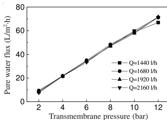
Fig. 2. Pure water flux as a function of transmembrane pressure for four different flow rates (Q) in the ultrafiltration membrane
