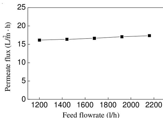
Fig. 6. Permeate flux variation as a function of feed flow rate in the ultrafiltration membrane (Transmembrane pressure =10 bar, temperature=30-35 °C, feed COD concentration = 3000 mg/L)
