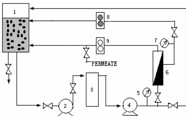
Fig. 1. Schematic diagram of ultrafiltration and nanofiltration membrane experimentation; 1. Tank, 2. Low-pressure pump, 3. Microfiltration membrane (Mf), 4. High-pressure pump, 5. Feed pressure gauge, 6. Uf Or Nf, 7. Concentrate pressure gauge, 8. Flow meter, 9. Flowmeter
