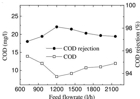
Fig. 13. Variation of COD and COD rejection with feed flow rate in the nanofiltration membrane (Transmembrane pressure = 10 bar, temperature = 30-35 °C, feed COD concentration = 570 mg/L, feed flow rate = 1440 L/h)
