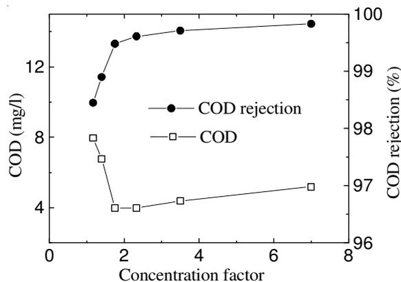
Fig. 15. Variation of COD and COD rejection with concentration factor in the nanofiltration membrane (Transmembrane pressure = 10 bar, feed flow rate = 1680 L/h, temperature = 30-35 °C, feed COD concentration = 570 mg/L, feed flow rate = 1440 l/h)
