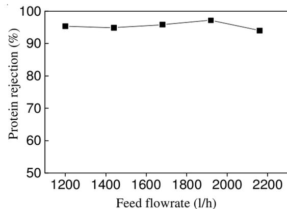
Fig. 7. Protein rejection as a function of feed flow rate in the ultrafiltration membrane (Transmembrane pressure =10 bar, temperature = 30-35 °C, feed COD concentration=3000 mg/L)
