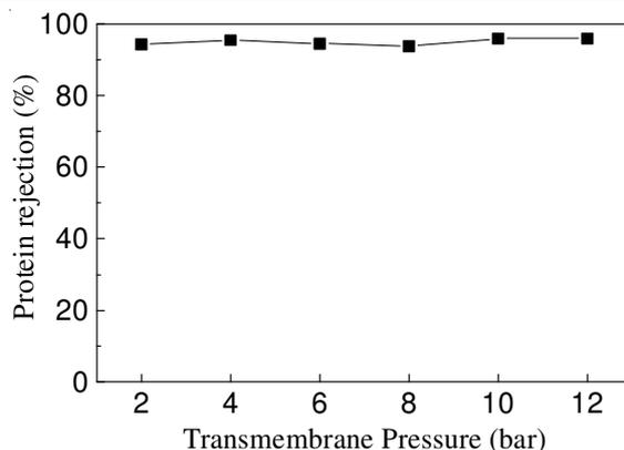
Fig. 5. Protein rejection as a function of transmembrane pressure in the ultrafiltration membrane (Feed flow rate =1440 l/h, temperature = 30-35 °C, feed COD concentration = 3000 mg/L)
