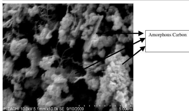
Fig. 19. SEM image of carbon nanotubes synthesized at 950 °C
