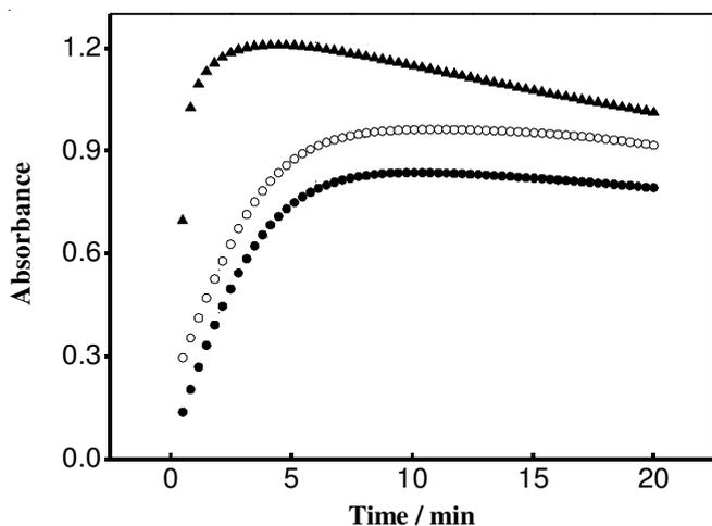
Fig. 4. Concentration of hemin and the relatively reaction time-response curves for  $\text{H}_2\text{O}_2$  detection. Experiment condition as follow,  $\text{H}_2\text{O}_2$ :  $1.0 \times 10^{-3}$  M, catechol:  $1.0 \times 10^{-4}$  M, hemin (●)  $1.5 \times 10^{-5}$  M, hemin (○)  $2.0 \times 10^{-5}$  M, hemin (▲)  $2.8 \times 10^{-5}$  M, temperature:  $35^\circ\text{C}$
