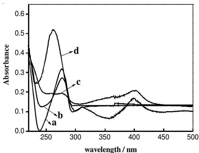
Fig. 1. UV-VIS absorption spectra of (a) catechol solution system (b) catechol and  $\text{H}_2\text{O}_2$  solution system (c) free hemin solution system (d) catechol- $\text{H}_2\text{O}_2$ -hemin system in aqueous-organic mixtures
