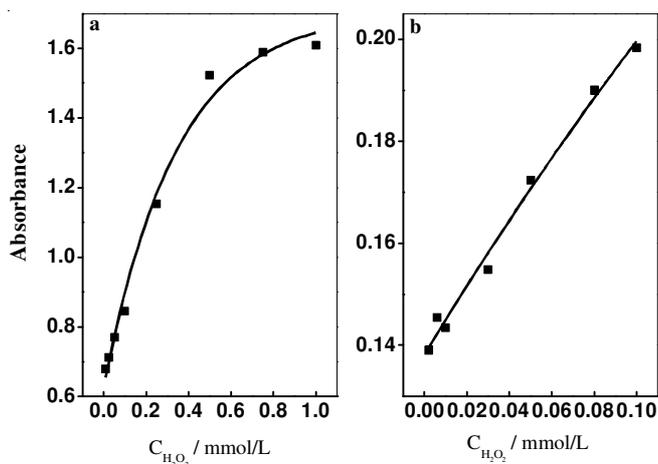
Fig. 5. (a) Concentration of  $\text{H}_2\text{O}_2$ -response curve for  $\text{H}_2\text{O}_2$  detection in aqueous-organic medium and (b) the calibration graph for the determination of  $\text{H}_2\text{O}_2$ . Hemin:  $1.9 \times 10^{-5}$  M, catechol:  $1.0 \times 10^{-4}$  M, temperature:  $35^\circ\text{C}$ , reaction time: 6 min
