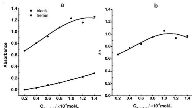
Fig. 2. (a) Concentration of catechol-response curves in the absence and presence of hemin; (b) The different concentration of catechol-A curve at 260 nm;  $\text{H}_2\text{O}_2$ :  $1.0 \times 10^{-3}$  M, hemin:  $2.8 \times 10^{-5}$  M, temperature:  $35^\circ\text{C}$ , reaction time: 5 min
