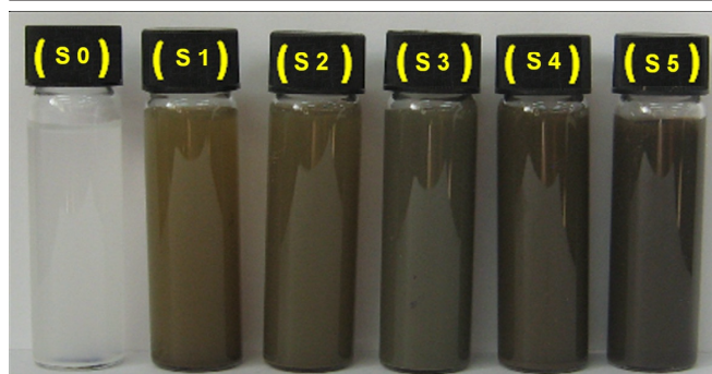
Fig. 1. Different range of Ag + /zeolite solution before and after addition of NaBH 4
