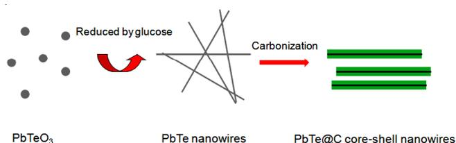
Fig. 6. Schematic illustration of formation of PbTe@carbon core-shell nanowires
