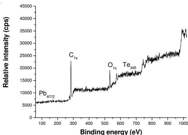
Fig. 3. XPS of the PbTe@carbon core-shell nanowires
