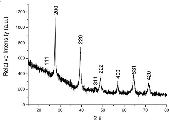
Fig. 5. XRD patterns of the as-prepared samples obtained from  $\text{Pb}(\text{OAc})_2 \cdot 3\text{H}_2\text{O}$  (0.0948 g, 0.25 mmol), 0.0553 g (0.25 mmol) of sodium tellurite and 1.5 g glucose in presence of 10 mL of PVA (3 wt %) solution at 160 °C for 4 h
