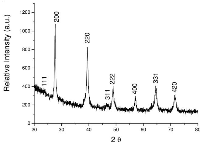
Fig. 1. XRD patterns of the as-prepared samples obtained from Pb(OAc)<sub>2</sub>·3H<sub>2</sub>O, sodium tellurite and glucose in presence of 10 mL of PVA (3 wt %) solution at 160 °C for 7 h
