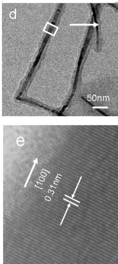
Fig. 2. (a-b) FESEM; (c-e) TEM images of the PbTe@carbon core-shell nanowires obtained from sodium tellurite, lead acetate and glucose in presence of PVA at 160 °C for 7 h
