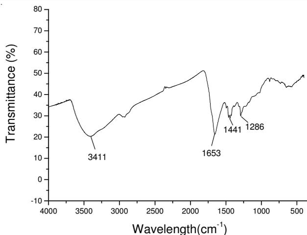
Fig. 4. FTIR spectrum of the PbTe@carbon core-shell nanowires
