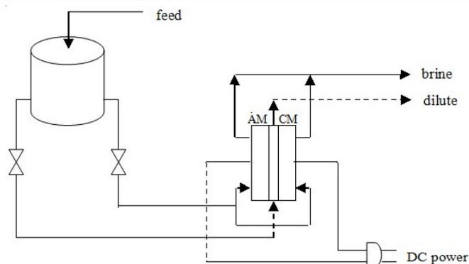
Fig. 3. Electro dialysis cell
