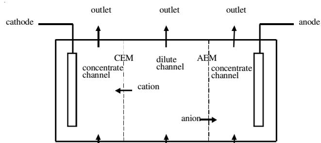
Fig. 2. Electro dialysis process principle
