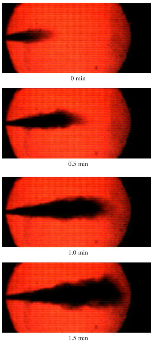
Fig. 4. Development process of the emulsion spray at ambient temperatures of 573 K and ambient pressure of 3.1 Mpa
