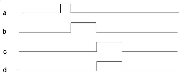
Fig. 2. Experimental process of the work of timing. a. Subscript signal; b. Trigger signal of single board computer; c. Suction signal of electromagnet; d. Trigger signal of high-speed camera and data acquisition system
