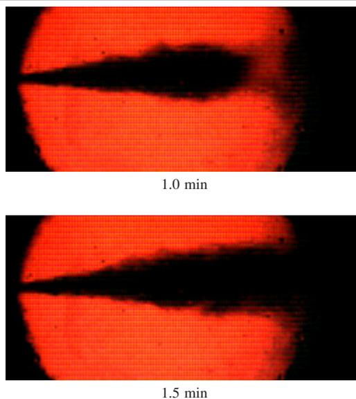
Fig. 3. Development process of the emulsion spray at ambient temperatures of 373 K and ambient pressure of 3.1 Mpa
