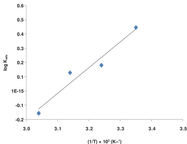
Fig. 4. Plots of  $\log K_{\text{ads}}$  against  $1/T$  for mild steel in absence and presence of different concentrations of *Ocimum basilicum* extract in 0.5M H<sub>2</sub>SO<sub>4</sub>
