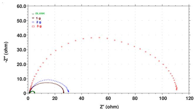
Fig. 6. Nyquist plots (EIS) of mild steel immersed in 0.5M  $\text{H}_2\text{SO}_4$  in absence and presence of different concentrations of *Ocimum basilicum* extract at 298 K
