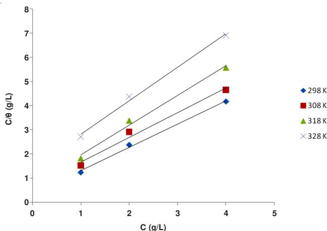
Fig. 3. Langmuir adsorption isotherm for adsorption of *Ocimum basilicum* extract on the surface of mild steel in 0.5M H<sub>2</sub>SO<sub>4</sub>
