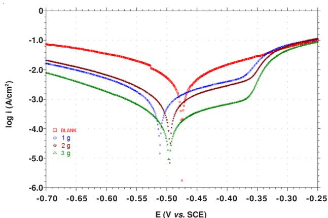
Fig. 1. Potentiodynamic polarization curves for mild steel in 0.5M H<sub>2</sub>SO<sub>4</sub> solution in absence and presence of different concentrations of *Ocimum basilicum* extract at 298 K
