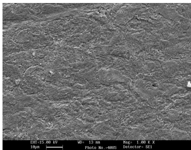
Fig. 7. (a) Scanning electron microgram of polished mild steel (1000  $\times$ ) after exposure to 0.5M  $\text{H}_2\text{SO}_4$ ; (b) Scanning electron microgram of polished mild steel (1000  $\times$ ) after exposure to 0.5M  $\text{H}_2\text{SO}_4$  containing 3 g of *Ocimum basilicum* extract
