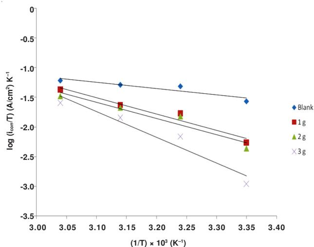
Fig. 5. Transition-state plots of  $\log(i_{\text{corr}}/T)$  versus  $1/T$  for mild steel corrosion in 0.5M  $\text{H}_2\text{SO}_4$  in absence and presence of various concentrations of *Ocimum basilicum* extract
