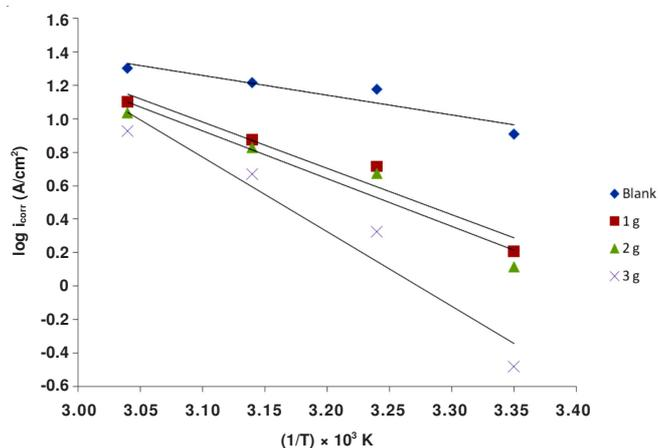
Fig. 2. Arrhenius plots of log i<sub>corr</sub> versus 1/T for mild steel corrosion in 0.5M H<sub>2</sub>SO<sub>4</sub> solution in absence and presence of different concentrations of *Ocimum basilicum* extract
