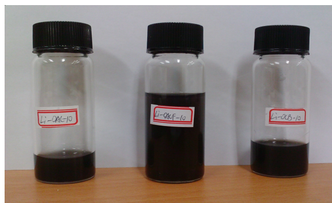
Fig. 3. Photographs of the typical Li treated carbon nanofluids (containing 10 wt % carbon materials (Li-OAC, Li-OACF, Li-OCB)) dispersed in distilled water
