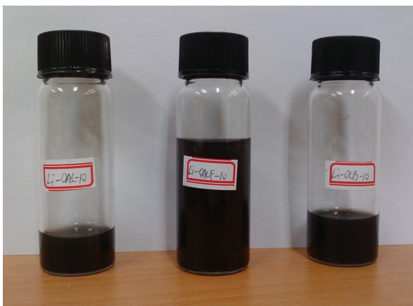
Fig. 1. Photographs of the Li treated carbon nanocolloids (containing 10 wt % carbon materials (Li-OAC, Li-OACF, Li-OCB)) dispersed in distilled water
