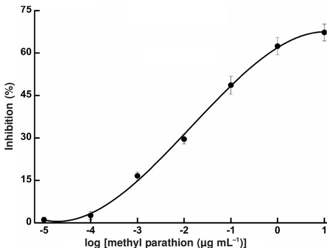
Fig. 6. Calibration curve for assaying methyl parathion using reconstituted AChE
