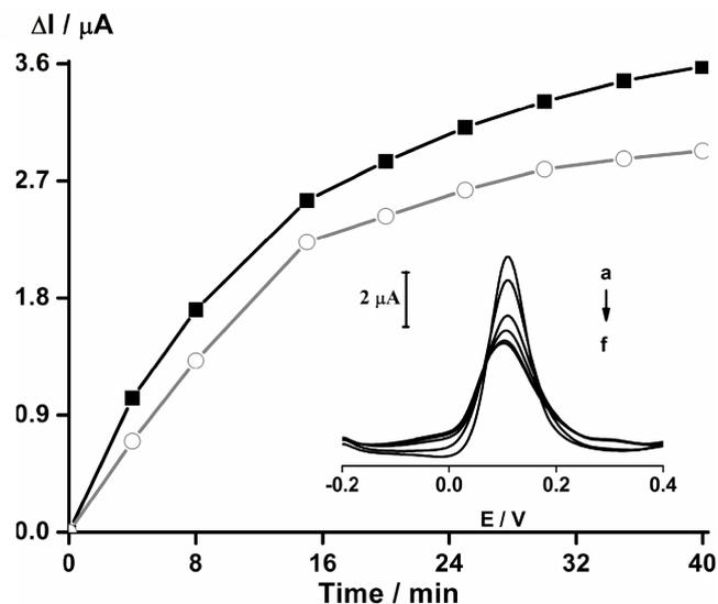
Fig. 1. The effects of enzymatic reaction time on the change of SWV peak values of 2,6-DCIP with (O): free AChE and (■): reconstituted AChE. The inset: SWV spectra of 2,6-DCIP with different enzyme reaction time (a) 0; (b) 4; (c) 8; (d) 15; (e) 20; (f) 25 min for free AChE. Potential step: 10 mV, amplitude: 25 mV and frequency: 10 Hz.
