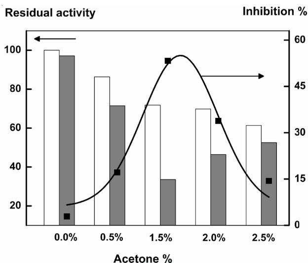
Fig. 5. Effect of acetone concentration on residual activity of reconstituted AChE and its inhibition efficiency by 1  $\mu\text{g}/\text{mL}$  methyl parathion in PBS containing acetone of different concentration for 10 min incubation
