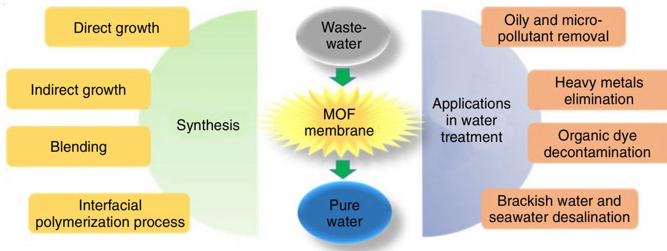
Fig. 1. Scheme summarizing synthetic procedures and applications of MOF based membranes in wastewater treatment
