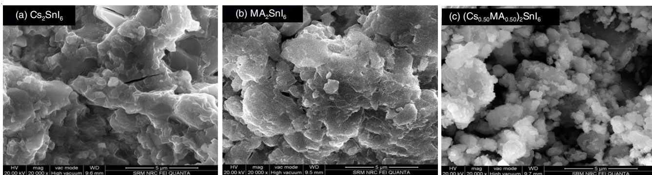
Fig. 6. FESEM images for synthesized double perovskite materials (a) \text{Cs}_2\text{SnI}_6 , (b) \text{MA}_2\text{SnI}_6 and (c) (\text{Cs}_{0.50}\text{MA}_{0.50})_2\text{SnI}_6
