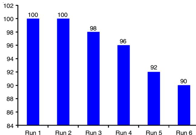
Fig. 3. Reusability test of the PC/AgNPs for model reaction
