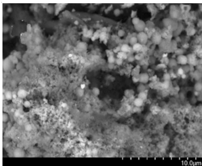
Fig. 1. SEM image of PC AgNPs (pH = 12.5, PC = 1 g, temperature = 80 °C, AgNO<sub>3</sub> = 6 mM) {Reprinted with permission [Ref. 35]}
