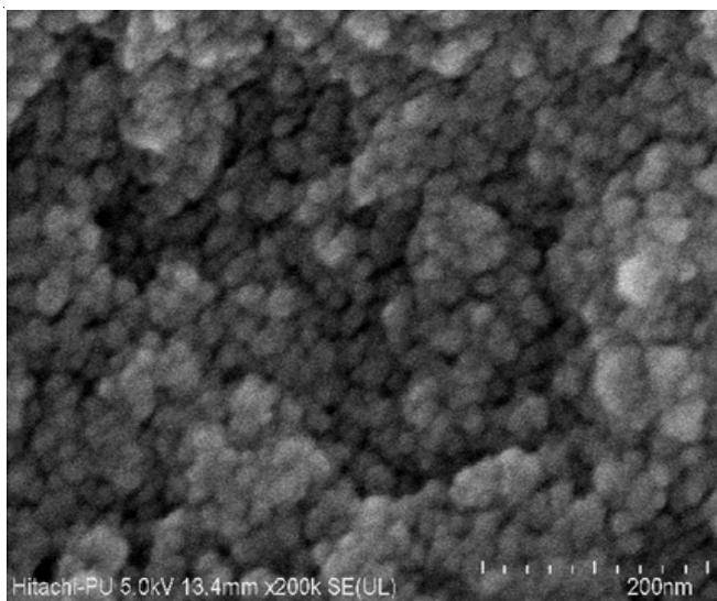
Fig. 2. FESEM of ZnO nanoparticles
