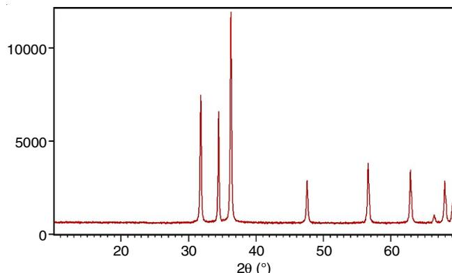
Fig. 3. XRD spectra of ZnO NPs
