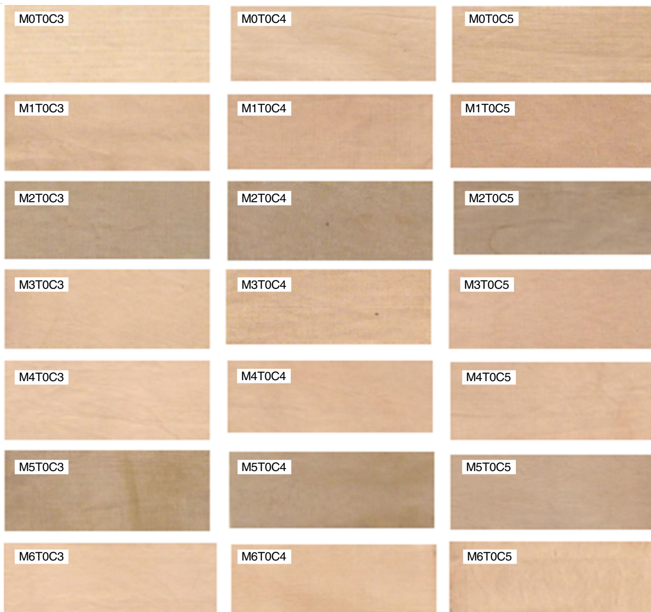
Fig. 5. Illustration of cotton fabrics dyeing by copperpod dye (M = mordant agent, T = Titania, C = immersion)
