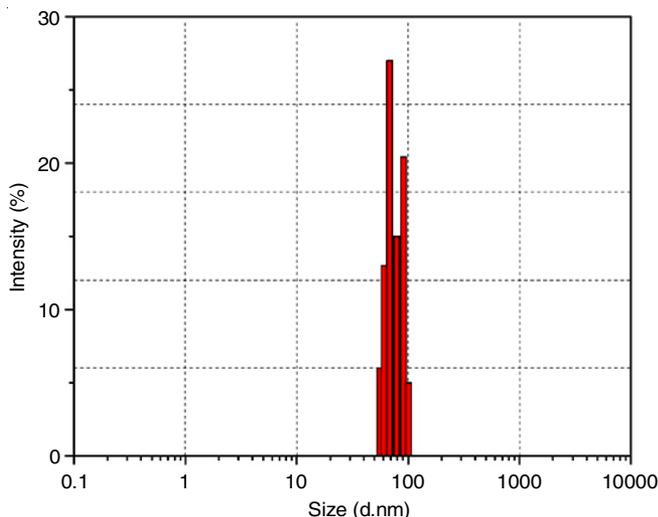
Fig. 3. DLS analysis of FeO nanoparticles
