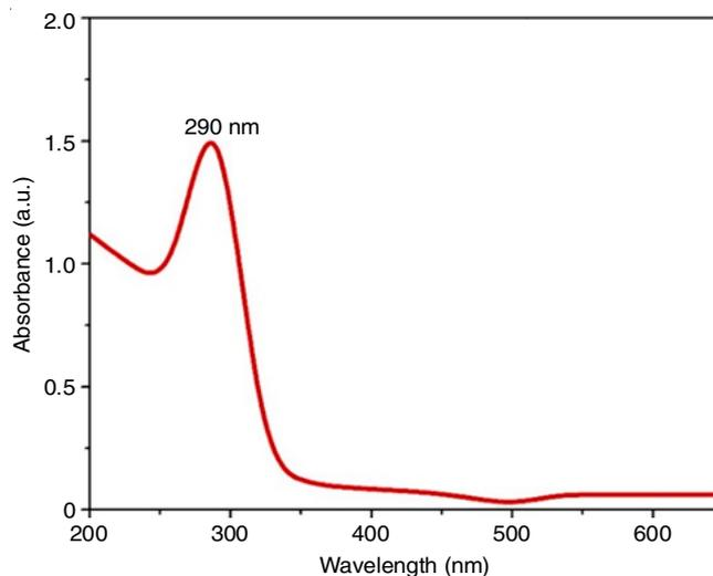
Fig. 1. UV-visible spectroscopic analysis of FeO nanoparticles
