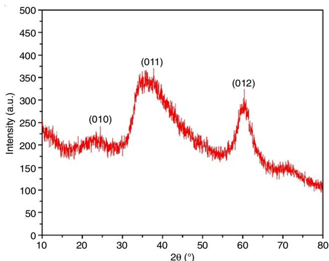
Fig. 2. XRD analysis of FeO nanoparticles
