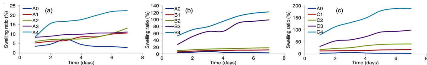
Fig. 6. Swelling ratio of (a) A blends, (b) B blends and (c) C blends
