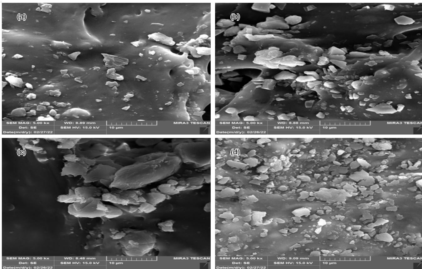
Fig. 4. FE-SEM of fracture tensile strength for (a) B1 blend, (b) B2 blend, (c) B3 blend, (d) B4 blend of (CH2)/NR
