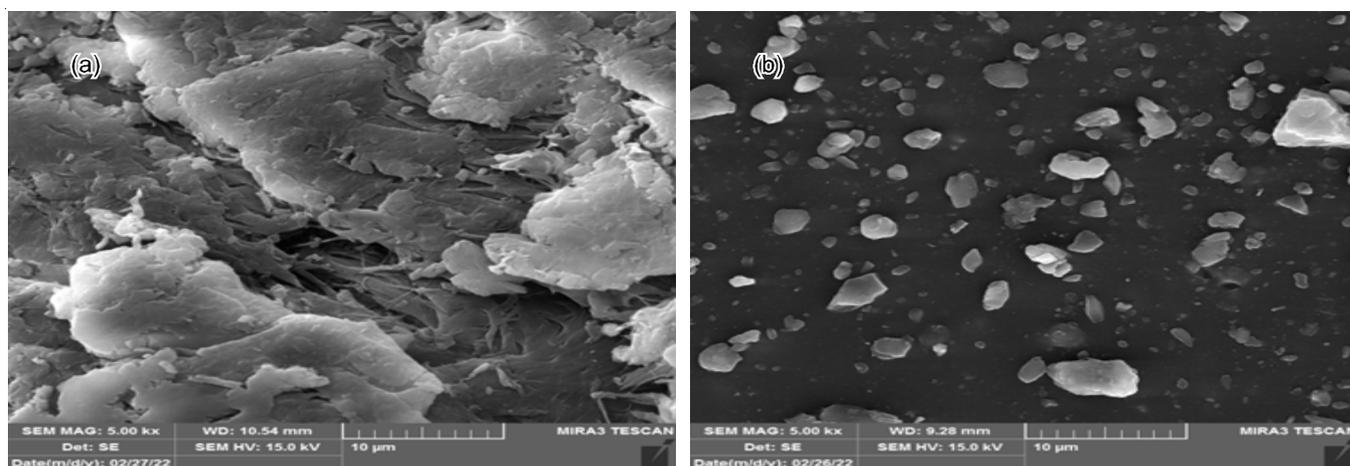
Fig. 2. FE-SEM of fracture tensile strength for (a) chitosan, (b) A0 blend
