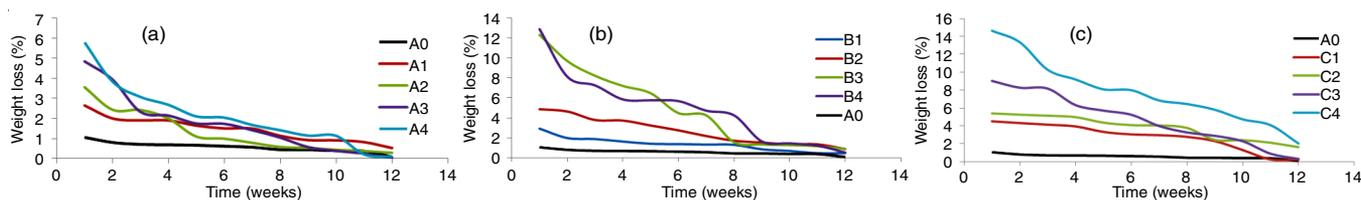
Fig. 9. Biodegradation of (a) A0, A1-4 blends in soil, (b) A0, B1-4 blends and (c) A0, C1-4 blends
