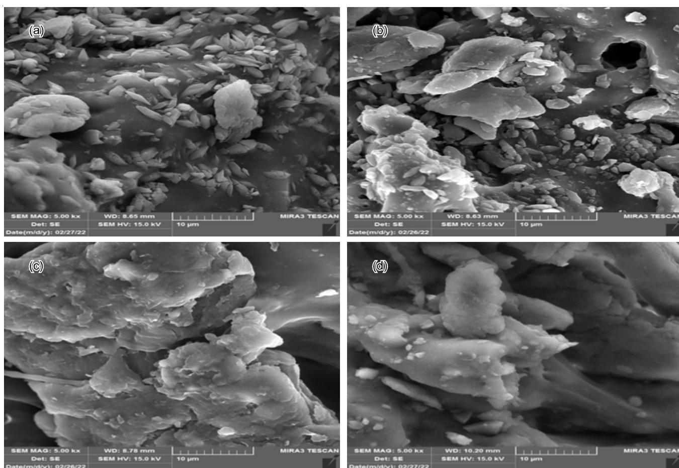
Fig. 3. FE-SEM of fracture tensile strength for (a) A1 blend, (b) A2 blend, (c) A3 blend, (d) A4 blend of (CH1)/NR
