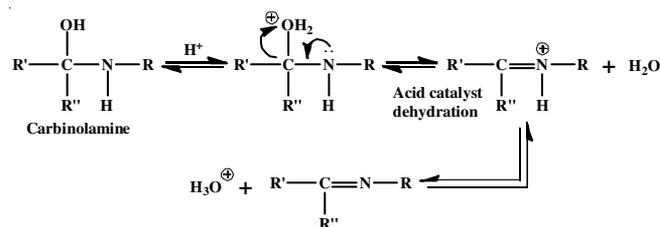
The loss of carbinolamine to water is the defining step of the limit reaction. In the proposed mechanism of the reaction of chitosan with amoxicillin, the carbonyl ketone group of amoxicillin with the primary amine group of chitosan react to form azomethine (-CH=N-) and eliminate a water molecule from the reaction by using the acid as catalyst.
