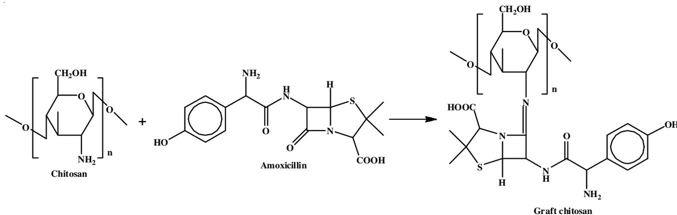
**Scheme-I:** Linking the compounds of the chitosan and recycled amoxicillin using condensation reaction
