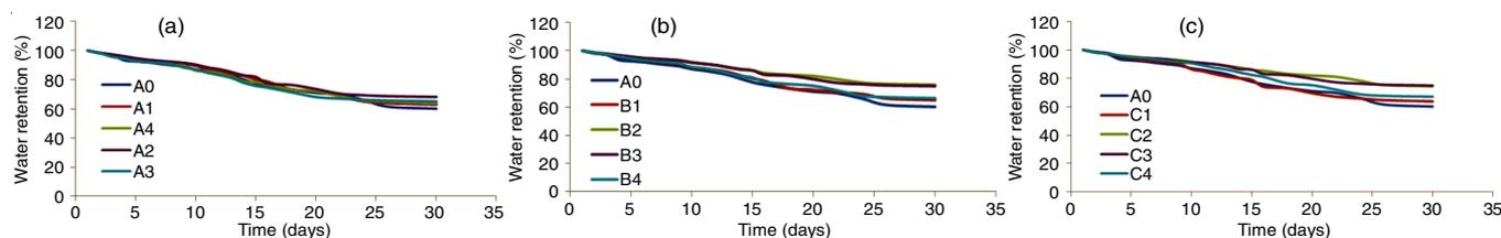
Fig. 7. Water retention of (a) A0, A blends in soil, (b) A0, B blends in soil (c) A0, C blends in soil
