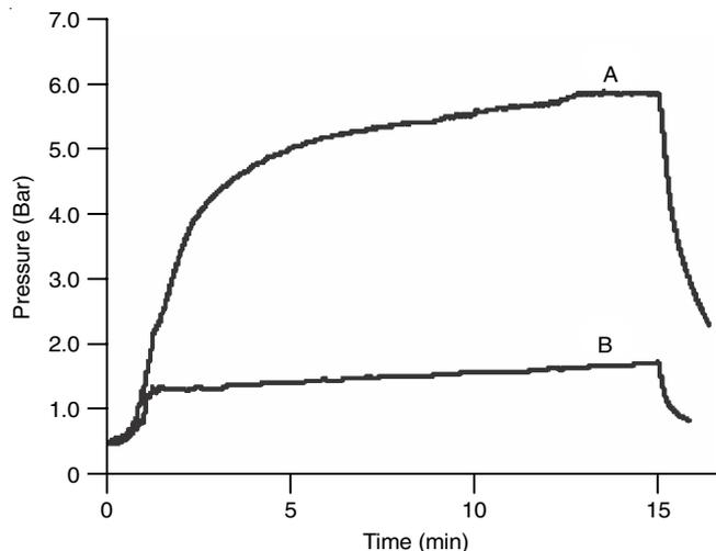
Fig. 1. Pressure-time curve observed from MW heating for 20 min: (A) solvent, base: (B) solvent, additive, substrate, catalyst and base
