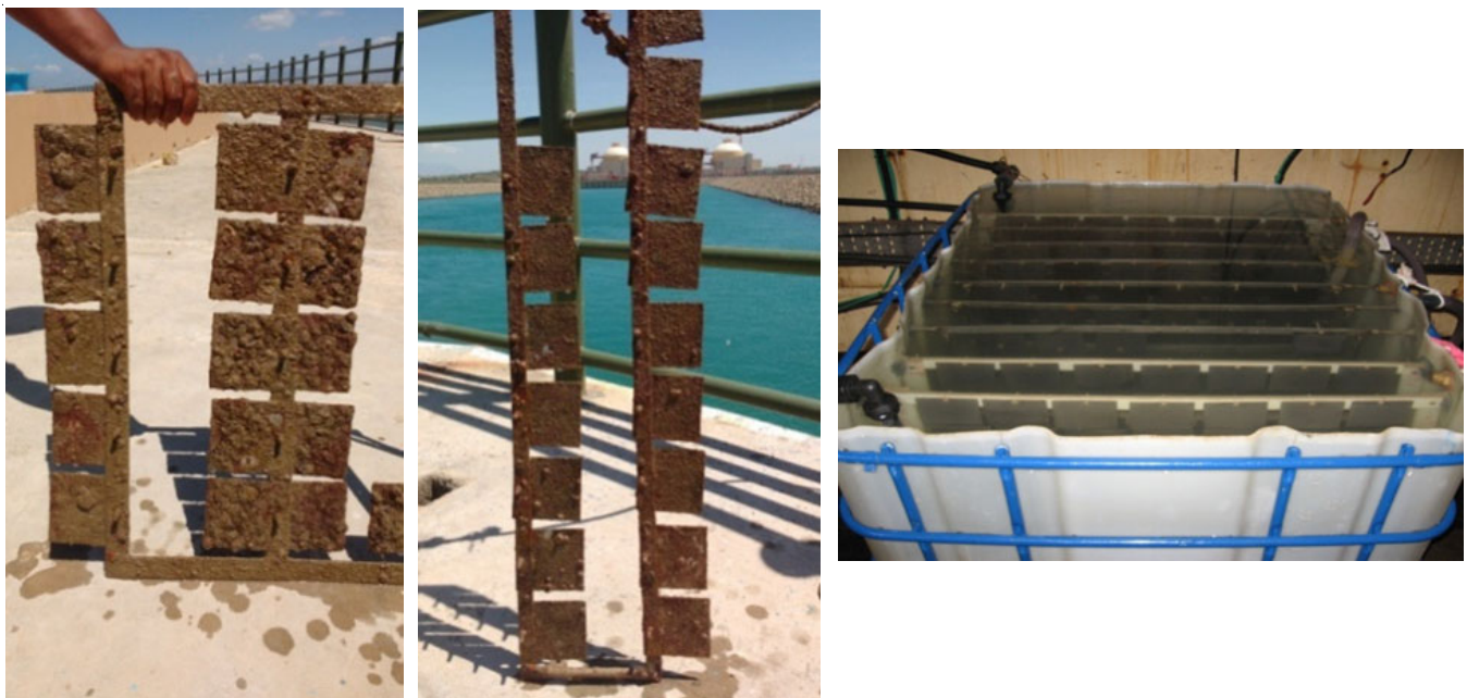
Fig. 4. Coupons deployed at the intake station and pump house station for long-term study
