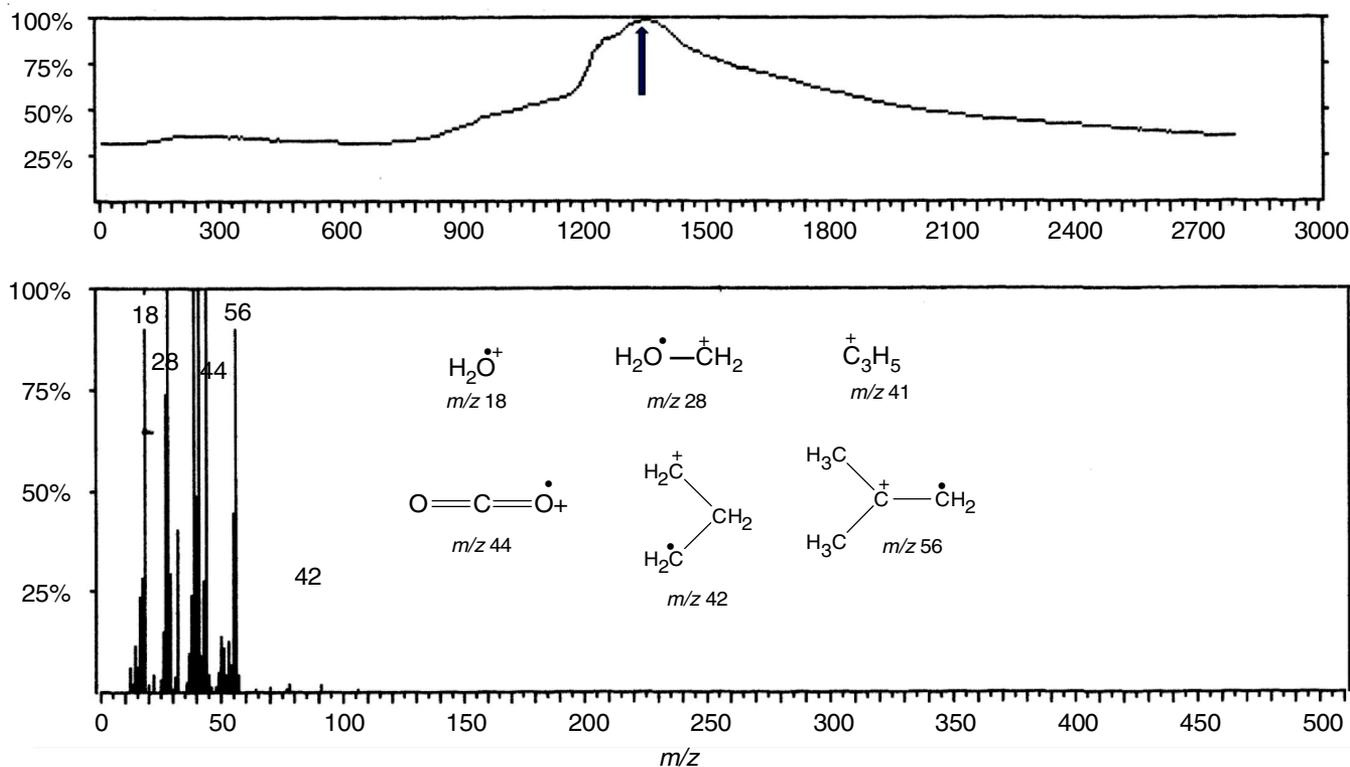
Fig. 9. Mass spectrometry of the gases emitted during the thermal reaction of Boc-Pro-Pro-Gly-OH (7) in the thermal analysis
