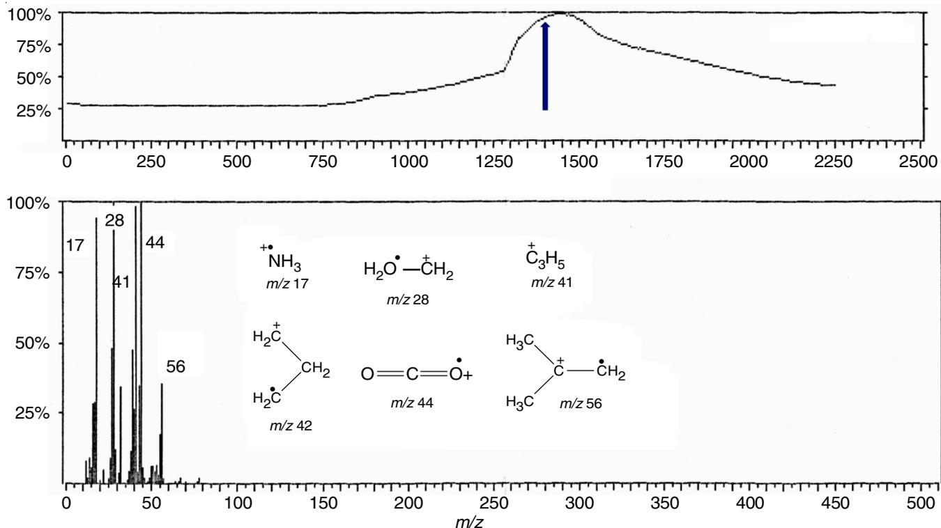
Fig. 10. Mass spectrometry of the gases emitted during the thermal reaction of Boc-Pro-Pro-Gly-NH<sub>2</sub> (8) in the thermal analysis
