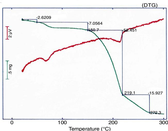
Fig. 7. TG (thermal gravimetry, green line) and DTA (differential thermal analysis, red line) of Boc-Pro-Pro-Gly-OH (7)
