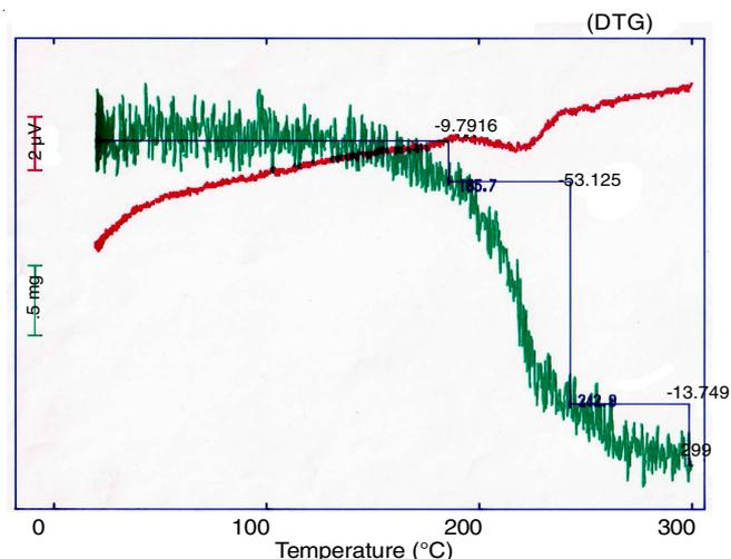
Fig. 8. TG (thermal gravimetry, green line) and DTA (differential thermal analysis, red line) of Boc-Pro-Pro-Gly-NH<sub>2</sub>·H<sub>2</sub>O (8)
