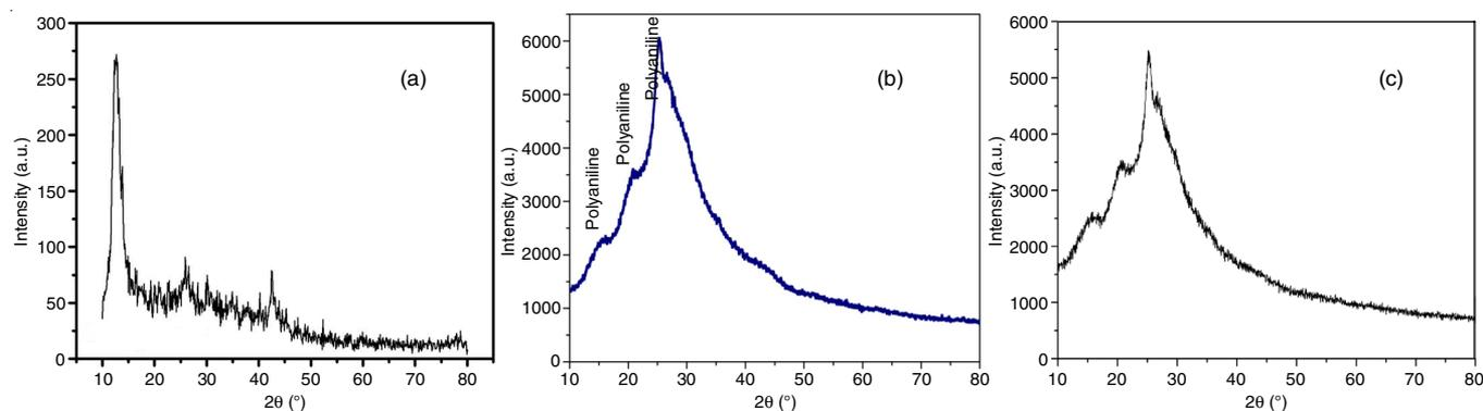
Fig. 2. XRD pattern of (a) GO nanocomposite, (b) polyaniline (PANI) and (c) PANI-GO nanocomposite 2 wt%
