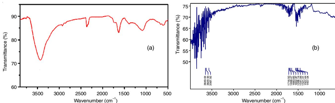
Fig. 3. FTIR spectra of (a) GO and (b) PANI/GO nanocomposite 2%wt
