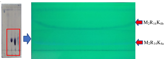
Fig. 5. TLC profile: (a) Five combined fractions of 90 fractions, (b) Preparative TLC of M_2R_{14}K_4 fraction
