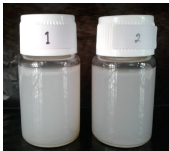
Fig. 1. Aqueous suspension of E. dulcis nanocellulose (1) hydrolysis for 60 min and (2) 120 min
