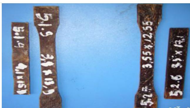
Fig. 2. Samples wood-HDPE composites for determining mechanical strengths
