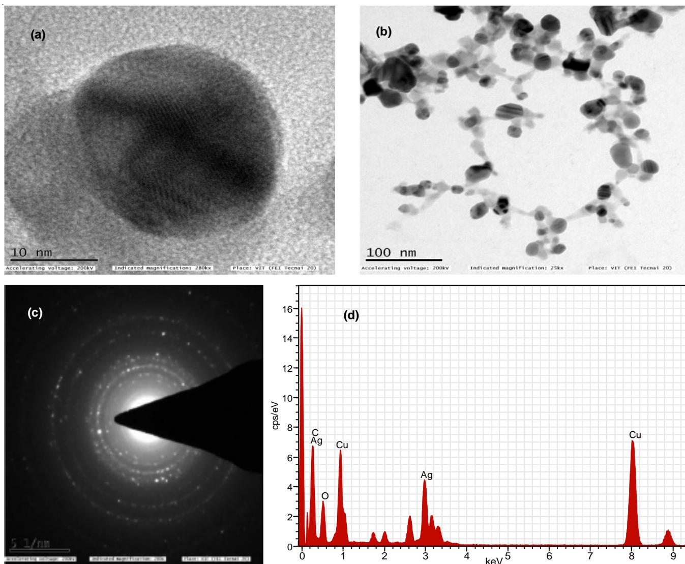
Fig. 3. (a&b) are the HR-TEM image of synthesized Cu-Ag NAs, (c) is the SAED diffraction pattern, (d) EDAX spectrum
