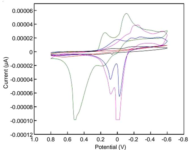
Fig. 4a. Cyclic voltammograms of bimetallic nanoparticle of colloidal media with different concentration 0.001 M, 0.005 M, 0.008 M, 0.01 M, 0.02 M at scan rate of 60 mV/s
