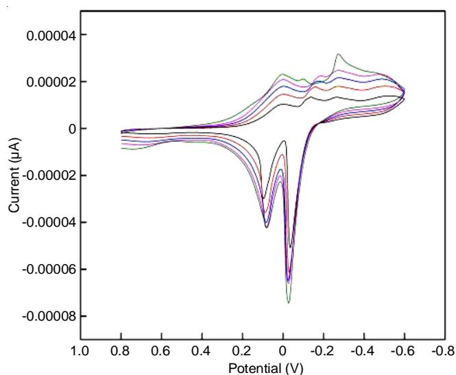
Fig. 4b. Cyclic voltammograms of bimetallic nanoparticle of colloidal media with different scan rate 20 to 100 mV/s at concentration of 0.008 M
