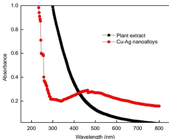
Fig. 1. UV-Visible spectrum of *Curcuma aromatica* plant extract and formed bimetallic Cu-Ag nanoalloys from the plant extract
