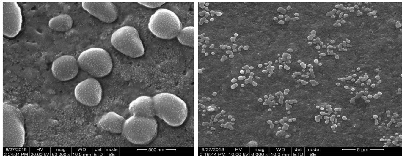
Fig. 2. FESEM images of Cu-Ag nanoalloy prepared at 80 °C from the plant extract
